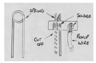
have been using Loctite gel which seems to give a good solid bond). Ensure that the spring wire goes across the end of the plunger tube and is in line. To prepare the plunger take the 2mm brass rod and screw it into the plunger jig level with the end. Cut of flush and file the end smooth. Still holding it in
