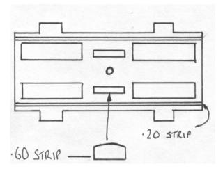
The bogies will require footboards and for this I used the plastic strip provided in the kit. Measure the distance between the bogies and cut the footboard strip to length. File a small curve on the outside corners and carefully scrape the edges round with the edge of a blade, then stick in place. I added small strips of .20 black plasticard to represent the brackets.
