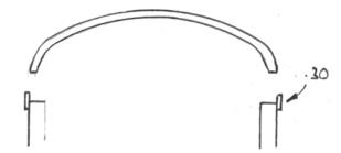
brake end coaches, because of the narrower brake end I had to glue the strip to the coach side for the corridor portion and then for the brake end glue the strip to the roof when it was finally cut to size and screwed in place. Remember to paint this strip teak when painting the side/roof.
